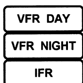
Fig. 2-24 This placard acc. to kind of operation airworthiness are located in direct pilot's view
