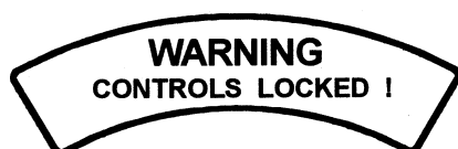
Fig. 2-26 This placard is located on the control stick locking latch
