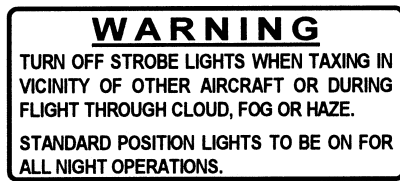
Fig. 2-28 This placard is located on the instrument panel (if strobe light installed)
