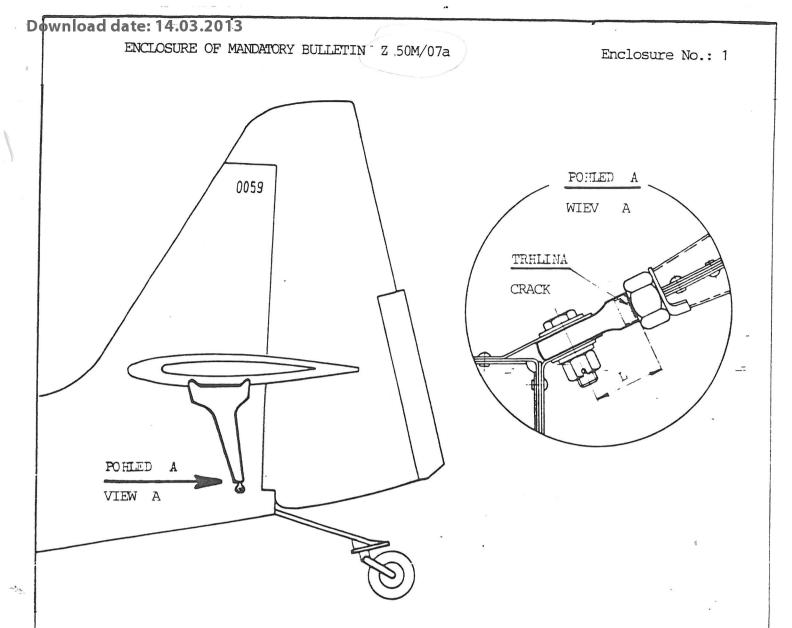
Check of the strut lower hinge eye (Valid for S/N 0078, 0079, 0080)
